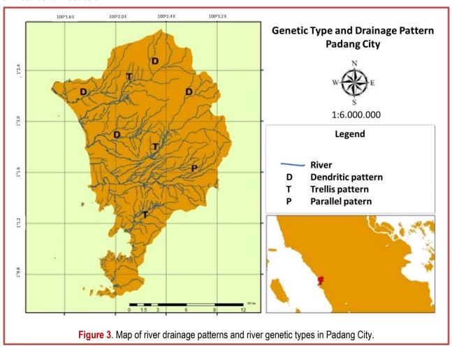
The drainage pattern seen in general in Padang City is dominated by dendritic (D), trellis (T), and parallel (P) drainage patterns. The results can be seen in Figure 3. The dendritic pattern tends to be in the north and west which is connected with a trellis patterned river in the middle to the south. While in the eastern area there is a parallel patterned river.
